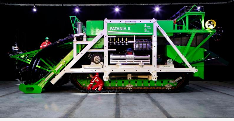
Figure 4 The Patania II which GSR is testing to collect nodules from the seabed in the CCZ Image: DEME Group: <u>https://www2.deme-group.com/</u>
