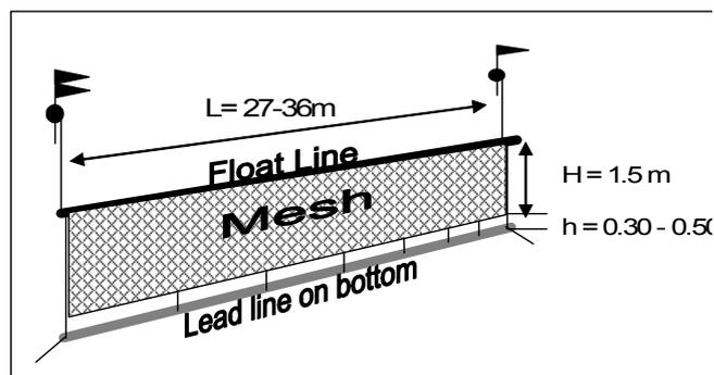
Fig. 1. Schematic model of the gill-net modification with "bottom escape windows" to reduce sturgeon by-catch in perch and pikeperch fisheries by using spacers between the bottom line and the lead line (detailed information on net characteristics are given in Table 1)
