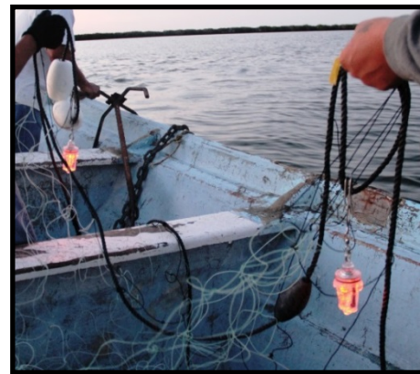
Figure 5.2.1: Orange LEDs attached to experimental gillnet.
