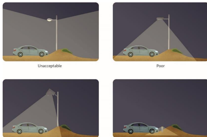
Figure 14 Lighting options for a parking area. © Pendoley Environmental, adapted from Witherington and Martin (2003) 3 .
