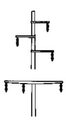
lines/wires should be spaced at least 140 cm apart. Hardware that is used to prevent arcing ("St. Elmo's fire" on both sides of the insulators) should not be used.
