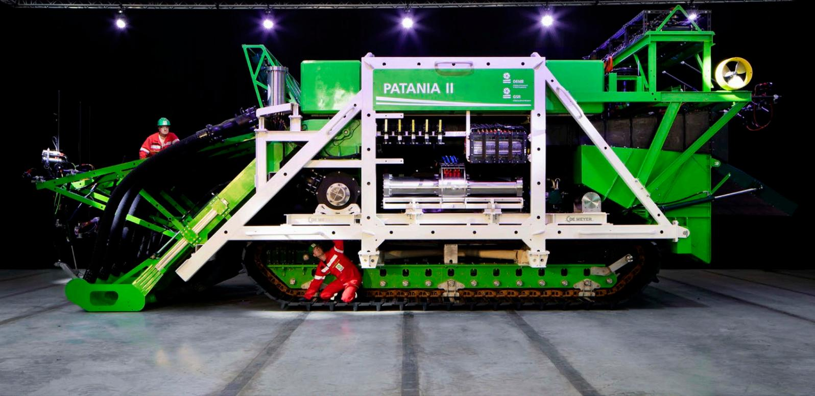
Figure 4 The Patania II which GSR is testing to collect nodules from the seabed in the CCZ
