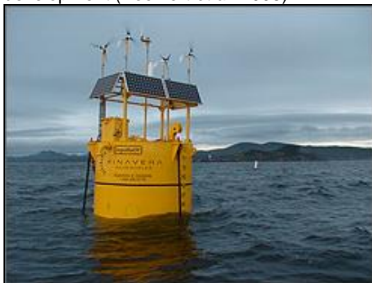
Buoy point absorber device. Image credit: US Dept. of Energy
