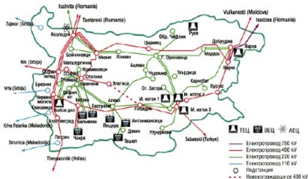
Figure 1. Bulgarian transmission network. Source: NEK (ABS Energy Research, 2011). The distribution network is not shown.
