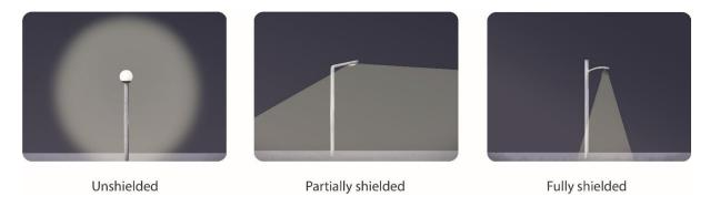
Figure 11 Lights should be shielded to avoid lighting anything but the target area or object.
