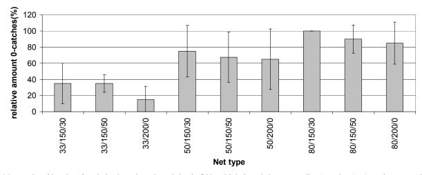
Fig. 5. Mean number of 0-catches of standard and experimental nets during the fishing trials in Szczecin Lagoon according (net code xx/yyy/zz reads as xx= mesh sizes (mm); yyy= height of mesh wall (cm); zz = height of bottom escape window (cm))
