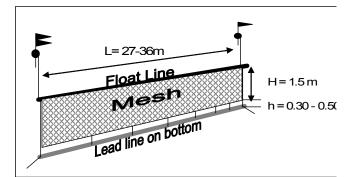
Fig. 1. Schematic model of the gill-net modification with "bottom escape windows" to reduce sturgeon by-catch in perch and pikeperch fisheries by using spacers between the bottom line and the lead line (detailed information on net characteristics are given in Table 1)
