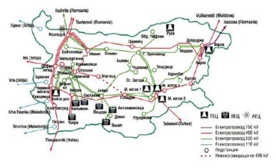
Figure 1. Bulgarian transmission network. Source: NEK (ABS Energy Research, 2011). The distribution network is not shown.
