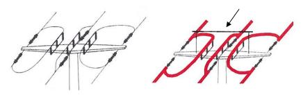
Figure 5. Left: Medium voltage pole with switch gear dangerous to perching birds because of short distances between energised parts. Right: Same pole after insulation of all energised wires close to the cross-arm (in red) and installing insulated safe perch (see arrow) (source: Haas et al., 2008).
