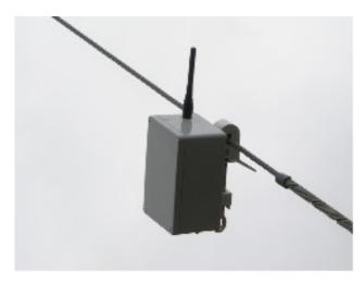
Figure 22. Bird Strike Indicator (BSI) attached to a power line. BSIs are relatively small devices that can be attached to a single wire of a power line and automatically register bird collisions based on the vibration of the wire.
