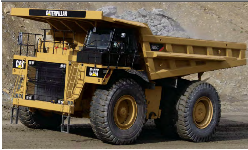
Figure 4.1 Example of a Caterpillar 785C Haul Truck (Capacity 140 tonnes per load)
