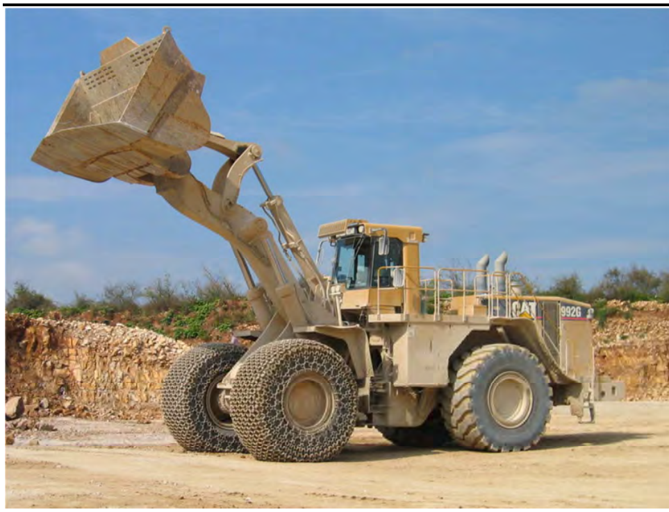
Figure 4.2 Example of a Caterpillar 992G Wheel Loader
