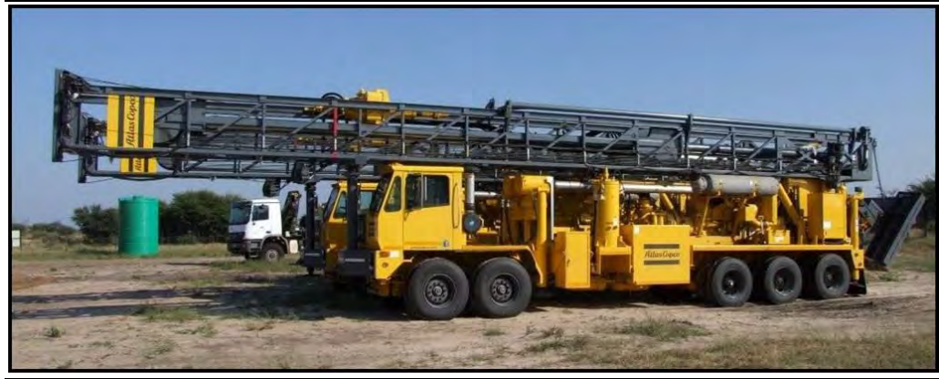
Figure 2.12 Example of an Atlas COPCO RD20 Oil and Gas Drilling Rig
